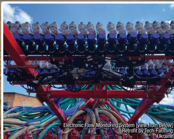
Elvorti seeder with flow indicators [top-right] fed to metering in-line check valves Ukraine
