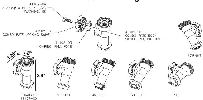
TO ADJUST ANGLE, LOOSEN SCREW AND ROTATE BODY AND THEN RE—TIGHTEN SCREW. THE ANGLE CAN BE ADJUSTED IN INCREMENTS OF 15° IN EITHER DIRECTION.
