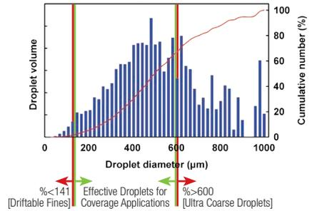
MR series is designed to produce relatively coarse spray with minimal drift.
