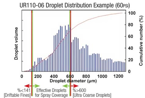
UR series is designed to produce ultra coarse spray with extremely little drift.
