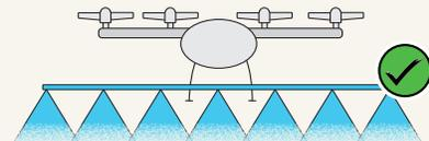
UAV sprayer applicators are able to use DX nozzles for targeted spray applications, but often due to boom constraints or UAV sprayer outfitting, wider angle nozzles like the MR110° nozzles might be used. In specialty circumstances that require a narrow full pattern spray can take advantage of the DX series of narrow-angle nozzles.
