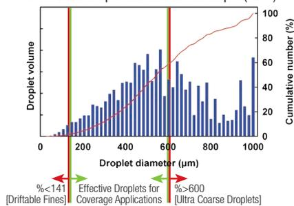
DR series is designed to produce extremely coarse spray with very minimal drift.
