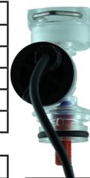
Each EFM (36 total) has a sensor cable plugged into it. When powered, each EFM sends signal through the Product Node Harness, to Product Node, to ECU.
