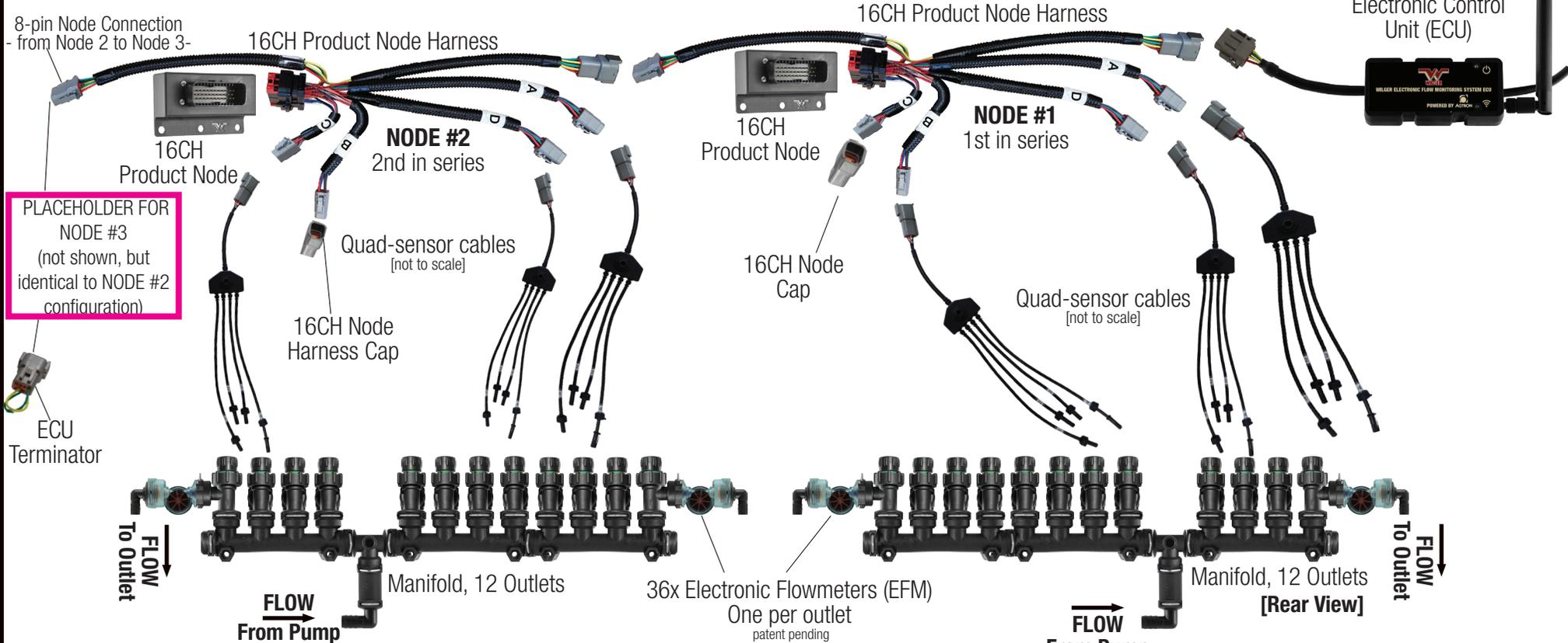
Electronic Flowmeters (EFM), Electronics & Harnesses Parts List
